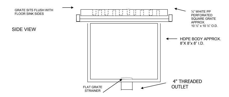
NOTE: ALL COMPONENTS ARE MADE OF ACID RESISTANT HDPE AND / OR PP MATERIALS.
