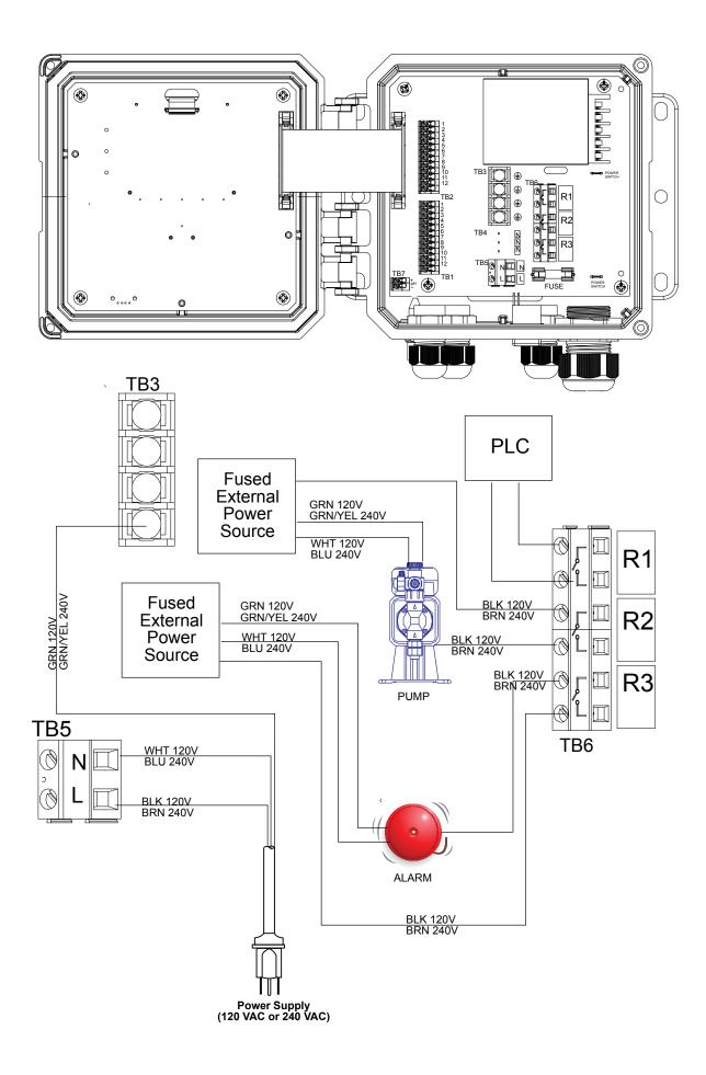
Figure 14 W110 AC Power & Relay Output Wiring
