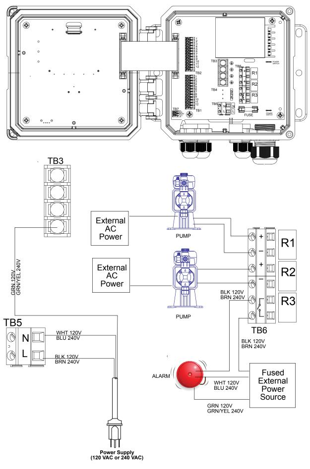
Figure 15 W120 AC Power & Relay Output Wiring
