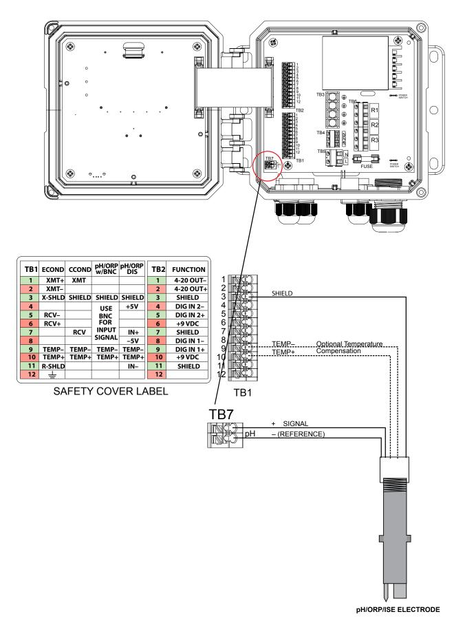
Figure 9 Non-Amplified pH/ORP/ISE Sensor Input Wiring
