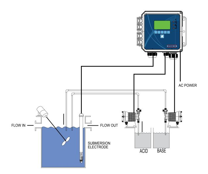
Figure 3 Typical Submersion Sensor Installation
