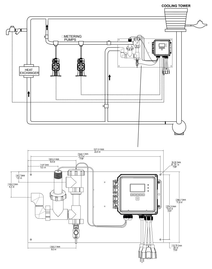
Figure 2 Typical Inline Sensor Installation
