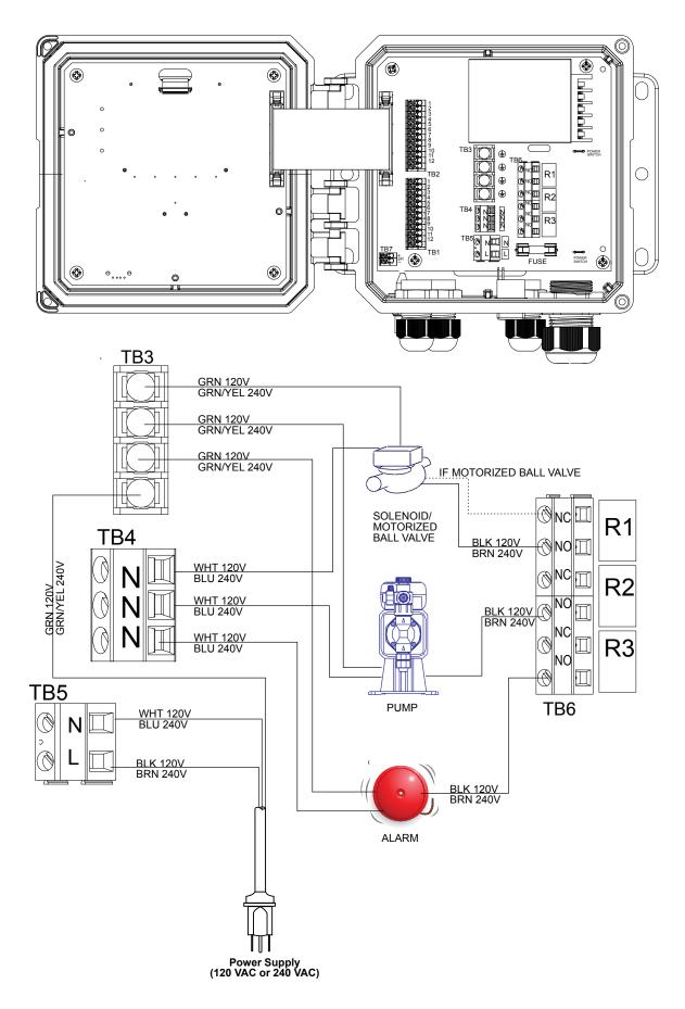
Figure 13 W100 AC Power & Relay Output Wiring
