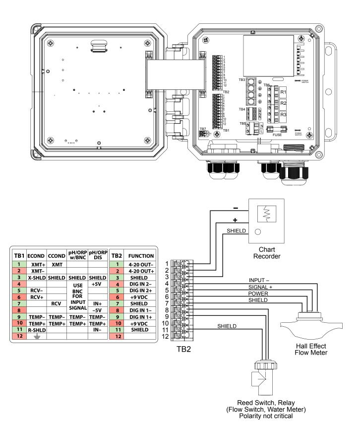
Figure 12 Digital Input /Analog Output Wiring
