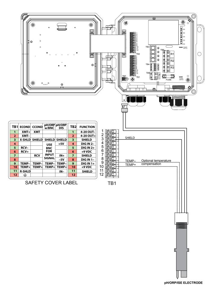
Figure 8 Non-Amplified pH/ORP/ISE Sensor Input Wiring with BNC
