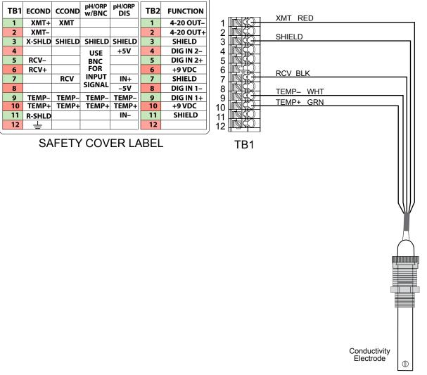
Figure 6 Contacting Conductivity Sensor Input Wiring
