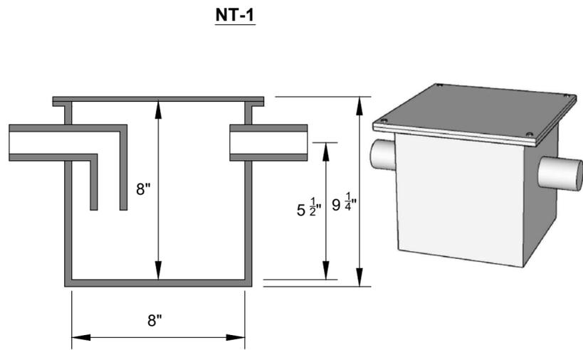
NT-1 IS A SIDE INLET AND OUTLET WITH BOLTED AND GASKETED COVER.
