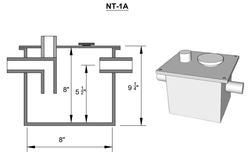
THE NT-1A HAS A CLEANOUT AND IS AVAILABLE WITH A TOP OR SIDE INLET AND SIDE OUTLET.
