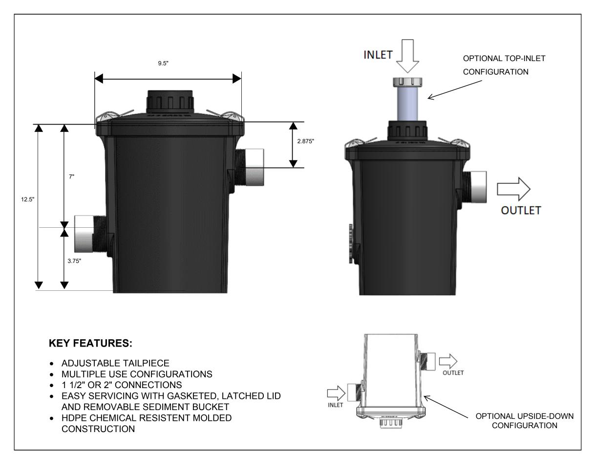
**Note:** Minimum of 5" is required above the SI-PC-150 for easy removal of sediment bucket.
