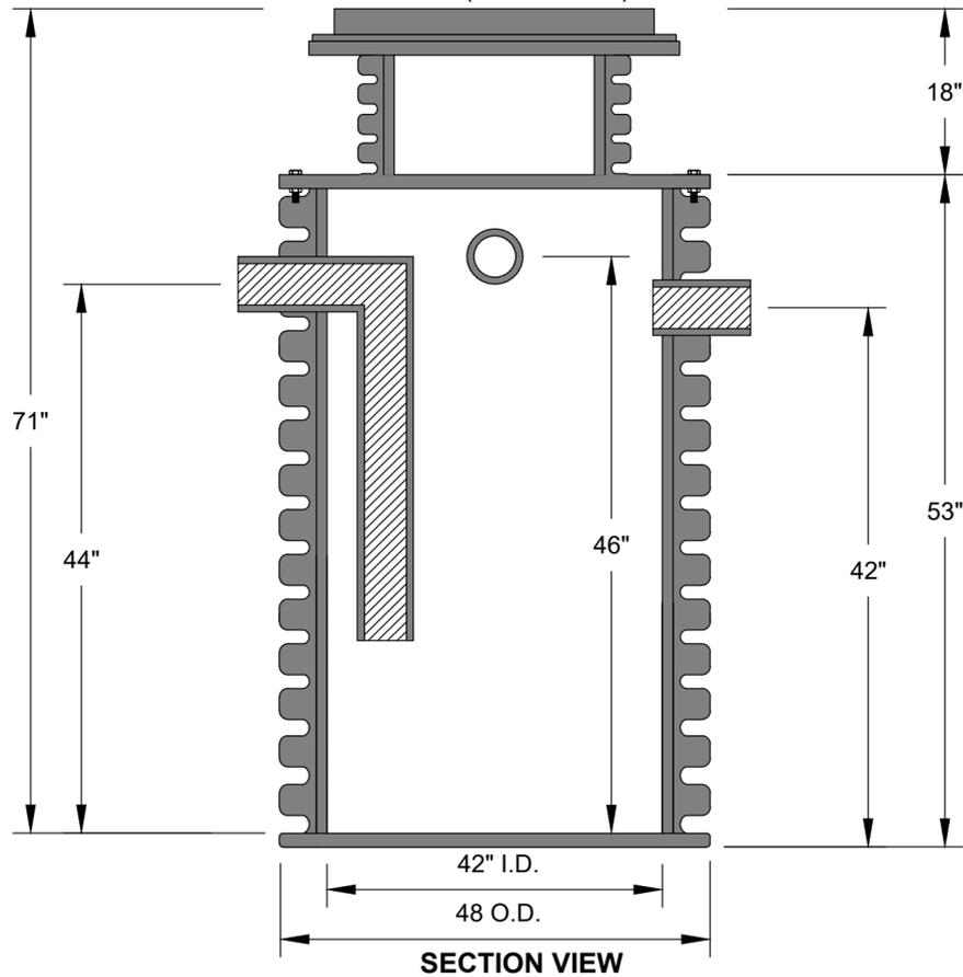
1" THICK PP COVER WITH RECESSED BOLTS FOR HEAVY DUTY PEDESTRIAN TRAFFIC WITH 18" FIELD ADJUSTABLE EXTENSION
